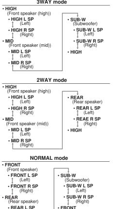
3-3. Push the [P.CH] button upward or downward to adjust "HIGH L SP", "HIGH R SP", "MID L SP", "MID R SP", "SUB-W L SP", "SUB-W R SP", "REAR L SP", "REAR R SP". "FRONT L SP" and "FRONT R SP".
